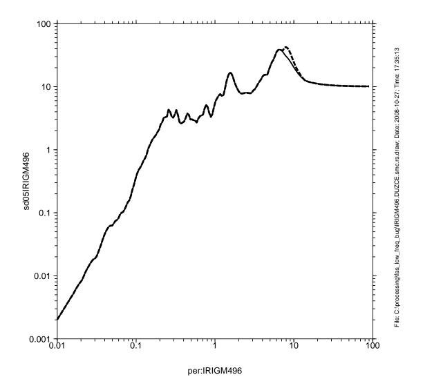
There will be a difference in the response spectra, although they must be the same at low and high periods (corresponding to PGA and PGD, respectively). This example suggests that blpadflt should be modified to add trailing zeros before causal filtering, but as we advocate acausal rather than causal filters, it may be awhile before I include that modification.
