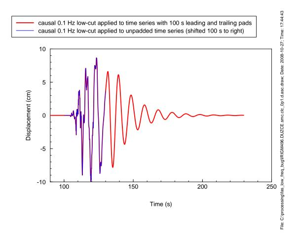
Clearly the peak displacement will be the same, but the unpadded time series will be missing a large amount of the filter transient. So even though there will be no difference in the portion of the time series corresponding to the original data, the FAS will be very different. But this being so, what about the response spectrum? A shown here
