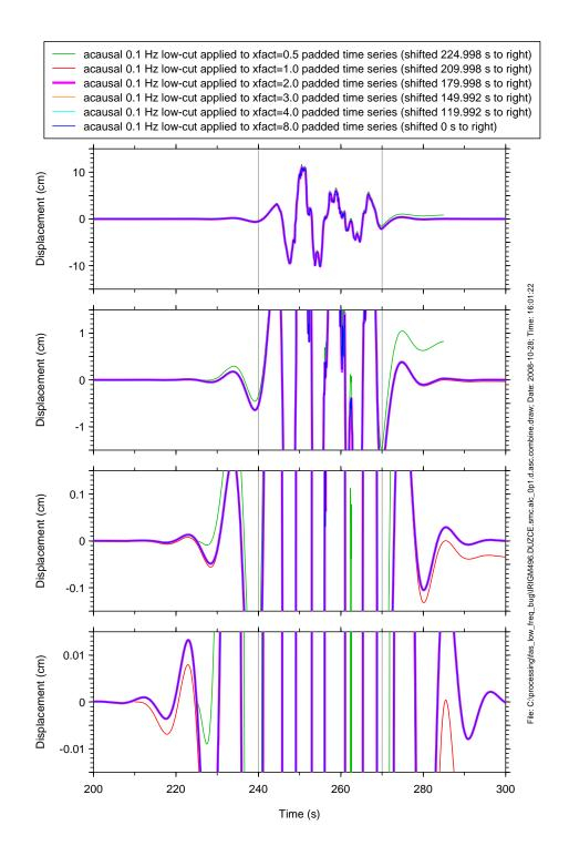
In these graphs the curves for  $xfact \ge 2.0$  are on top of one another. The vertical gray lines indicate the duration of the original time series. The horizontal is the same for all graphs. As best seen in the lower two graphs, there are small differences between the standard case and the cases with a longer duration of added pads; these small differences show up in the FAS at low frequencies.
