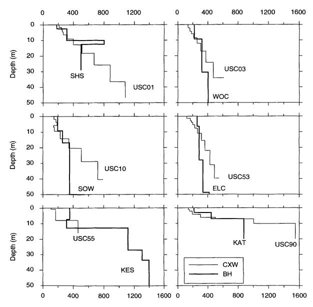
▲ Figure 5 (corrected). Shear-wave velocity profiles obtained from the CXW method at six USC sites (thin lines), compared with velocities from downhole velocity profiles in boreholes drilled at or near the USC sites (thick lines).
