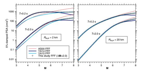
**Figure 2.** Pseudospectral acceleration (PSA) versus moment magnitude (**M**) for the ACR model described in the E electronic supplement, using the finite-fault factors (FFF) shown in Figure 1. The results are shown for rupture distances ( $R_{RUP}$ ) of 2 and 20 km and periods (T) of 0.2 and 2.0 s. The color version of this figure is available only in the electronic edition.
