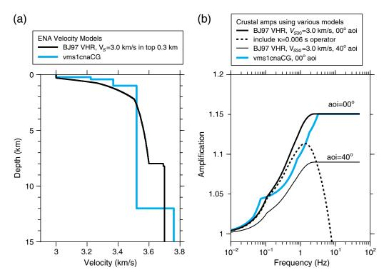
**Figure 5.** (a) Velocity models for a very-hard-rock (VHR) site in eastern North America (ENA): vms1cnaCG and the modified Boore and Joyner (1997; BJ97). See text for an explanation of the models. (b) Amplifications for the two models; the amplification for the BJ97 model is shown for two angles of incidence (aoi), without and with the attenuation operator for aoi = 00°. The color version of this figure is available only in the electronic edition.
