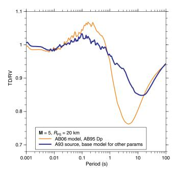
**Figure 9.** Ratios of response spectra from TD and RV simulations for two of the models used in Figure 8, for M = 5.0 and  $R_{\rm PS} = 20$  km. (a) The model parameters are given in the electronic supplement. The color version of this figure is available only in the electronic edition.
