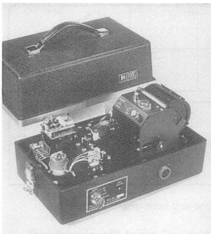
Fig. 1. Typical strong-motion recording instrument, which records three components of ground motion on photographic film. (Photo from Kinematics).
