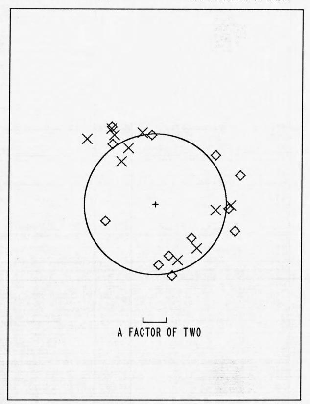
Figure 45. Peak horizontal velocity in the San Fernando earthquake recorded at the base of small structures. Azimuthal dependence of the residuals from the mean regression line. See
