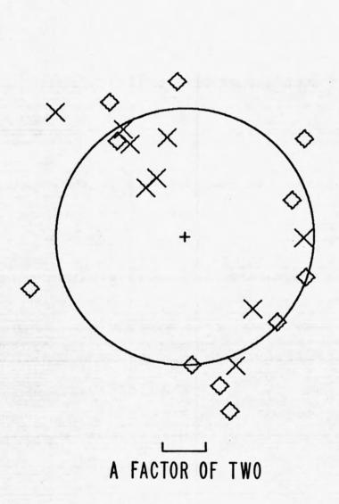
Figure 46. Peak horizontal displacement in the San Fernando earthquake recorded at the base of small structures. Azimuthal dependence of the residuals from the mean regression line. See text for further explanation. Symbols same as in Figure 1.
