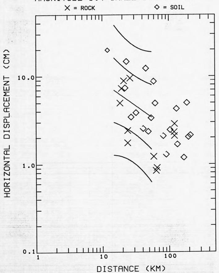
Figure 11. Peak horizontal displacement versus distance to the slipped fault for the magnitude range 7.1-7.7 recorded at the base of small structures. Symbols same as in Figure 1.
