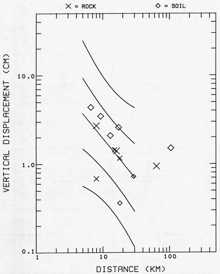
Figure 21. Peak vertical displacement versus distance to the slipped fault for magnitude 6.4 recorded at the base of small structures. Symbols and curves same as in Figure 1.
