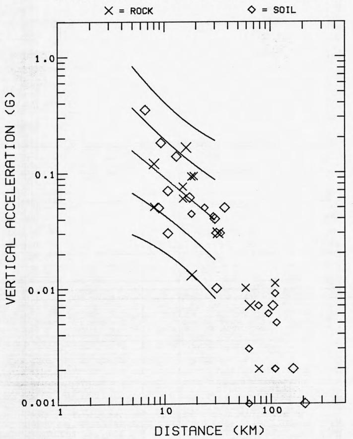
Figure 15. Peak vertical acceleration versus distance to the slipped fault for the magnitude range 6.0-6.4 recorded at the base of small structures. Symbols and curves same as in Figure 1.
