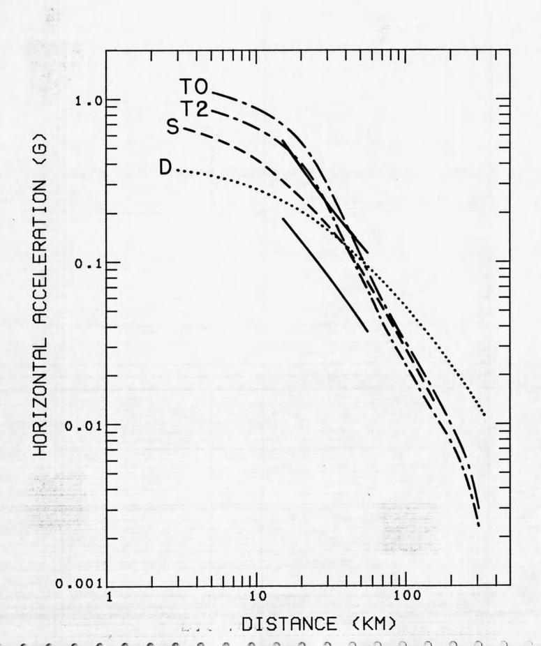
Figure 48. Proposed relationships for peak horizontal acceleration from a magnitude 7.6 earthquake. Curves labeled S, D, TO and T2 are from the sources given in Figure 41. The solid lines show the 70 percent prediction interval for the small-structure magnitude 7.1-7.7 data set of this report.
