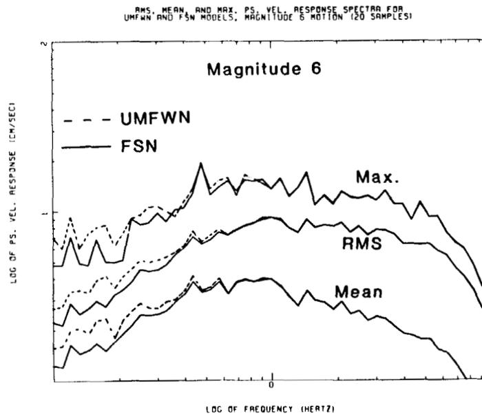
Figure 6. Maximum, mean and RMS pseudo-velocity response spectra calculated from UMFVN and FSN models for magnitude 6 earthquake
