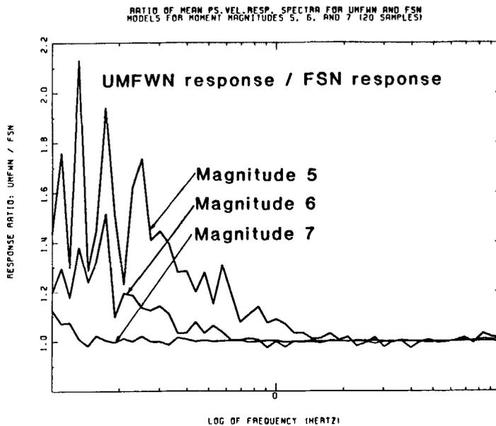
Figure 8. Ratio of pseudo-velocity response spectra due to UMFWN model to that due to FSN model for magnitudes 5, 6 and 7
