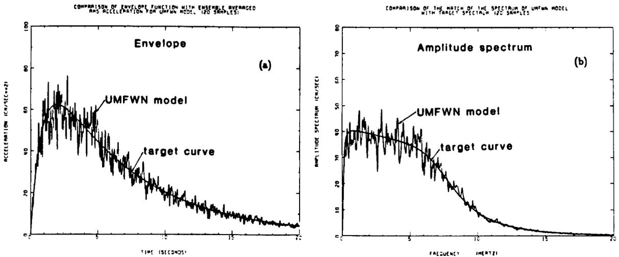
Figure 2. Match of the simulation with target values for magnitude 7 earthquake, UMFWN model, 20 samples: (a) ensemble average of the envelope function; (b) ensemble average of the Fourier amplitude spectra
