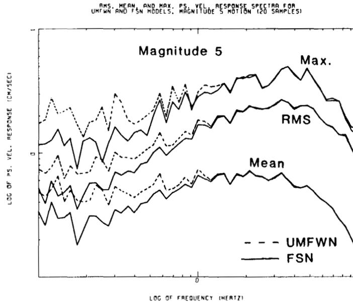
Figure 5. Maximum, mean and RMS pseudo-velocity response spectra calculated from UMFVN and FSN models for magnitude 5 earthquake
