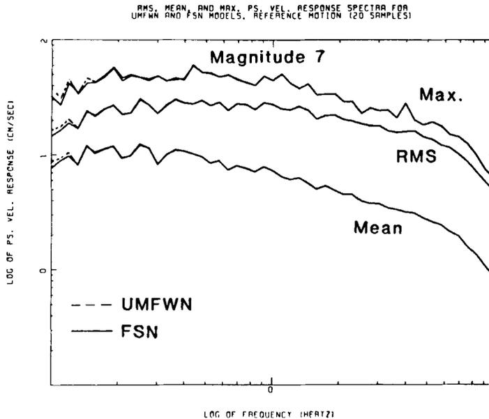
Figure 7. Maximum, mean and RMS pseudo-velocity response spectra calculated from UMFWN and FSN models for magnitude 7 earthquake
