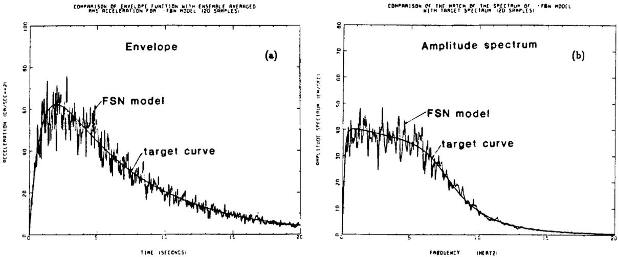
Figure 3. Match of the simulation with target values for magnitude 7 earthquake, FSN model, 20 samples: (a) ensemble average of the envelope function; (b) ensemble average of the Fourier amplitude spectra
