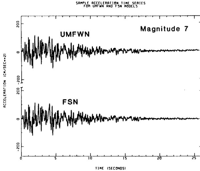
Figure 1. A sample of acceleration time series generated by UMFWN and FSN models for magnitude 7 earthquake
