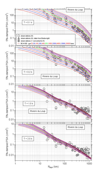
**Figure 2.7** Observations from the 2005 Riviere du Loup earthquake (symbols) and simulated PSA for a suite of stress parameters, using crustal amplifications for  $V_{S30} = 2.0$  km/sec and the Boore et al. [2010] (BCA10D) attenuation model. See Boore [2012] for details regarding the observations.
