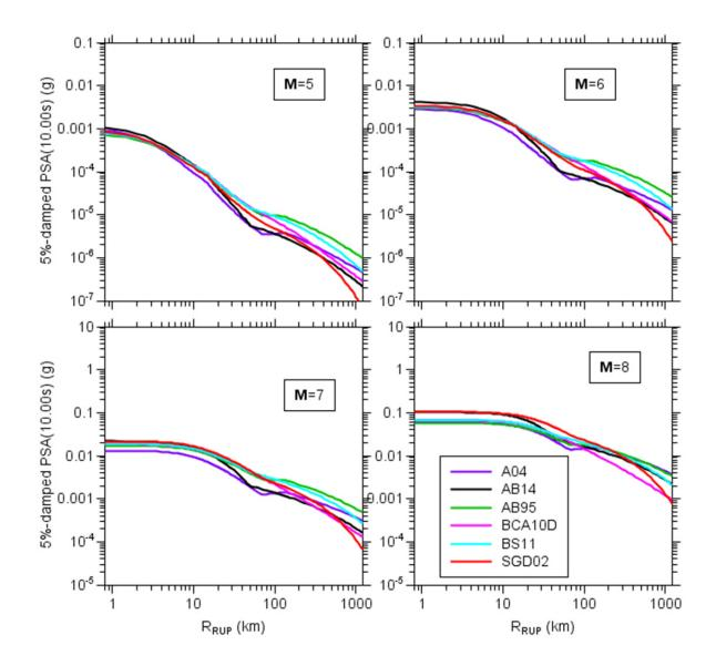
Figure 2.17 A comparison of simulated 5%-damped response spectra from the six attenuation models for a period of 10.0 sec as a function of distance for four magnitudes. The crustal amplifications used in the simulations were for sites with  $V_{s30} = 3.0$  km/sec.
