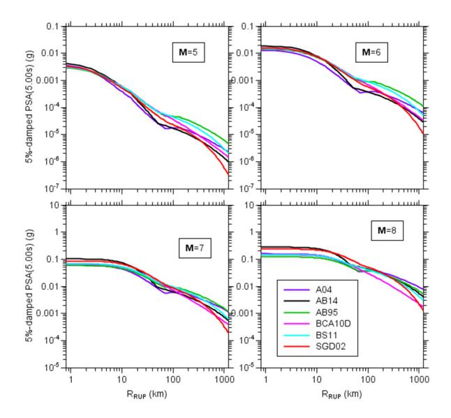
Figure 2.16 A comparison of simulated 5%-damped response spectra from the six attenuation models for a period of 5.0 sec as a function of distance for four magnitudes. The crustal amplifications used in the simulations were for sites with  $V_{s30} = 3.0$  km/sec.
