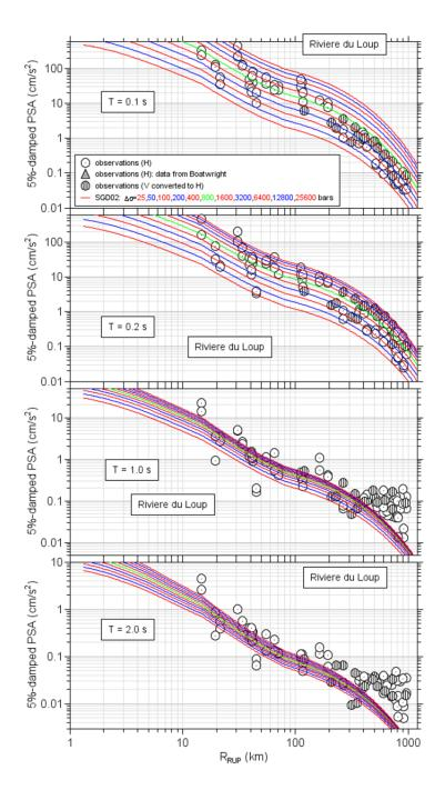
**Figure 2.9** Observations from the 2005 Riviere du Loup earthquake (symbols) and simulated PSA for a suite of stress parameters, using crustal amplifications for  $V_{S30} = 2000$  m/sec and the Silva et al. [2002] (SGD02) attenuation model. See Boore [2012] for details regarding the observations.
