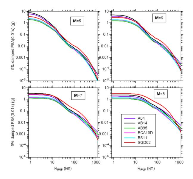
Figure 2.11 A comparison of simulated 5%-damped response spectra from the six attenuation models for a period of 0.01 sec as a function of distance for four magnitudes. The crustal amplifications used in the simulations were for sites with  $V_{s30} = 3.0$  km/sec.
