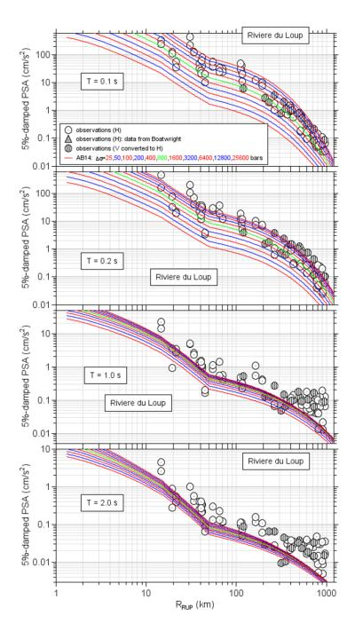
**Figure 2.5** Observations from the 2005 Riviere du Loup earthquake (symbols) and simulated PSA for a suite of stress parameters, using crustal amplifications for  $V_{S30} = 2.0$  km/sec and the Atkinson and Boore [2014] (AB14) attenuation model. See Boore [2012] for details regarding the observations.
