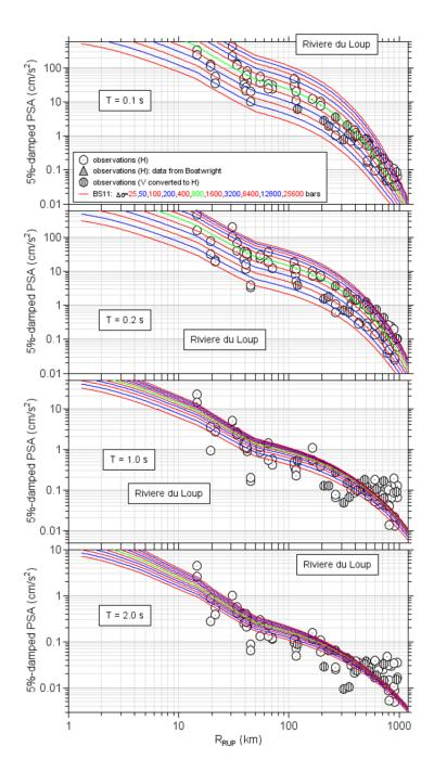
**Figure 2.8** Observations from the 2005 Riviere du Loup earthquake (symbols) and simulated PSA for a suite of stress parameters, using crustal amplifications for  $V_{s30} = 2.0$  km/sec and the Boatwright and Seekins [2011] (BS11) attenuation model. See Boore [2012] for details regarding the observations.
