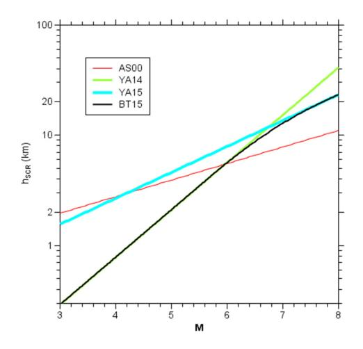
**Figure 2.3** The finite-fault (FF) factor  $h_{SCR}$  (where "SCR" stands for "stable continental region") used in converting the closest distance to the rupture surface  $(R_{RUP})$  to the distance to be used in the point-source calculations
