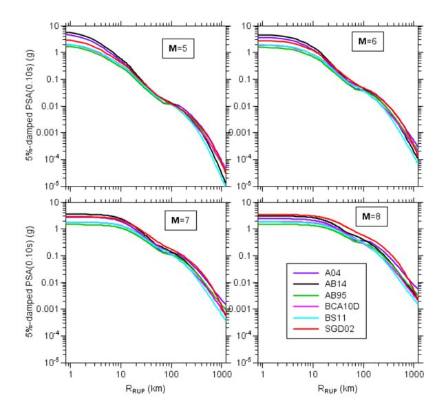
Figure 2.12 A comparison of simulated 5%-damped response spectra from the six attenuation models for a period of 0.1 sec as a function of distance for four magnitudes. The crustal amplifications used in the simulations were for sites with  $V_{s30} = 3.0$  km/sec.
