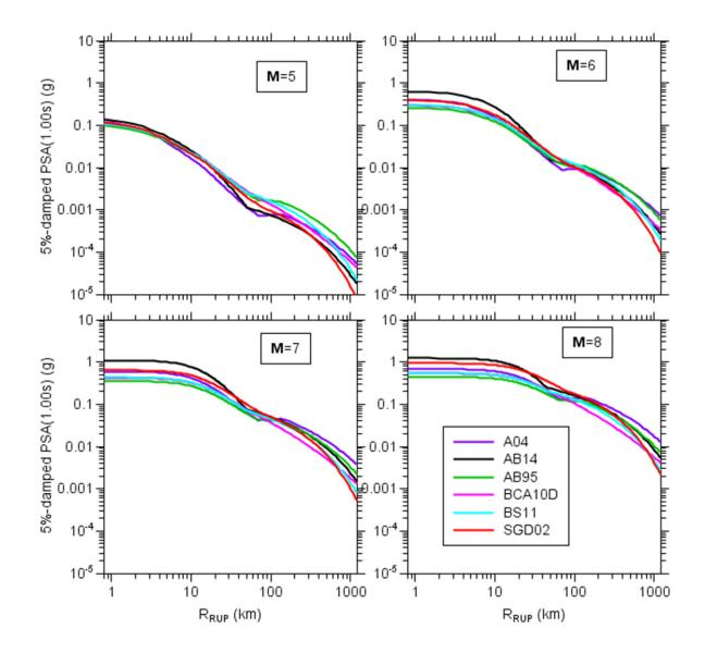
Figure 2.14 A comparison of simulated 5%-damped response spectra from the six attenuation models for a period of 1.0 sec as a function of distance for four magnitudes. The crustal amplifications used in the simulations were for sites with  $V_{s30} = 3.0$  km/sec.
