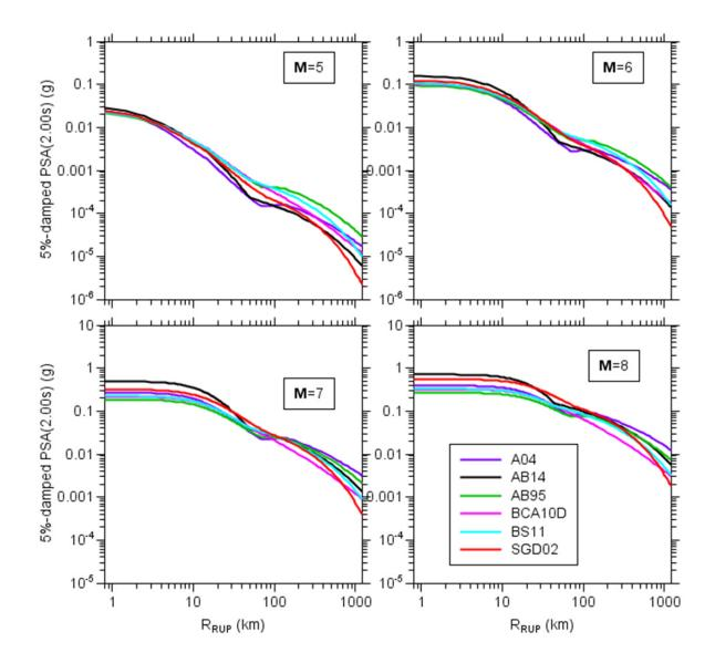
Figure 2.15 A comparison of simulated 5%-damped response spectra from the six attenuation models for a period of 2.0 sec as a function of distance for four magnitudes. The crustal amplifications used in the simulations were for sites with  $V_{s30} = 3.0$  km/sec.
