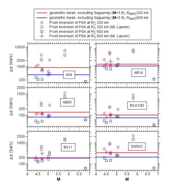
**Figure 2.10** Summary of stress parameters obtained from inversions of observed PSA for the six attenuation models. The results from inversions using data within 200 km and within 600 km are shown separately. The stress parameters from recording of the Mt. Laurier earthquake are shown as separate symbols to distinguish those results from the other event (Kipawa) with the same M.
