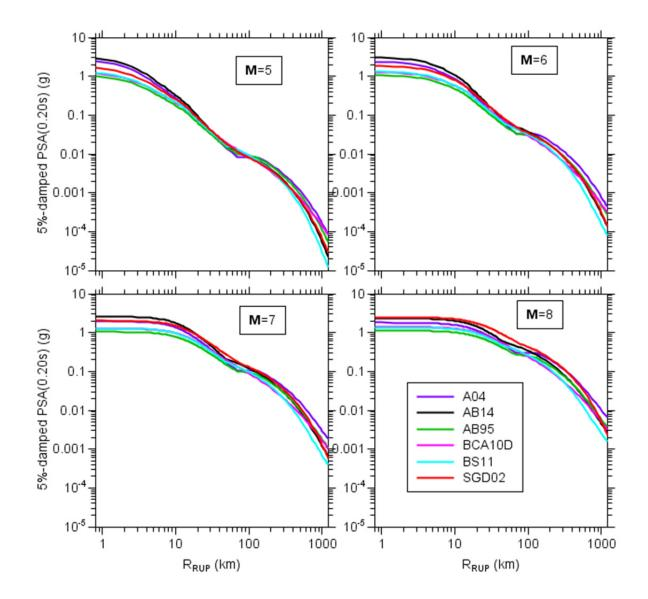
Figure 2.13 A comparison of simulated 5%-damped response spectra from the six attenuation models for a period of 0.2 sec as a function of distance for four magnitudes. The crustal amplifications used in the simulations were for sites with  $V_{s30} = 3.0$  km/sec.
