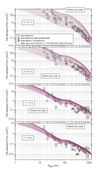
**Figure 2.6** Observations from the 2005 Riviere du Loup earthquake (symbols) and simulated PSA for a suite of stress parameters, using crustal amplifications for  $V_{S30} = 2.0$  km/sec and the Atkinson and Boore [1995] (AB95) attenuation model. See Boore [2012] for details regarding the observations.
