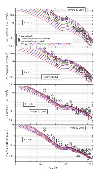
**Figure 2.4** Observations from the 2005 Riviere du Loup earthquake (symbols) and simulated PSA for a suite of stress parameters, using crustal amplifications for  $V_{s30} = 2.0$  km/sec and the Atkinson [2004] (A04) attenuation model. See Boore [2012] for details regarding the observations.
