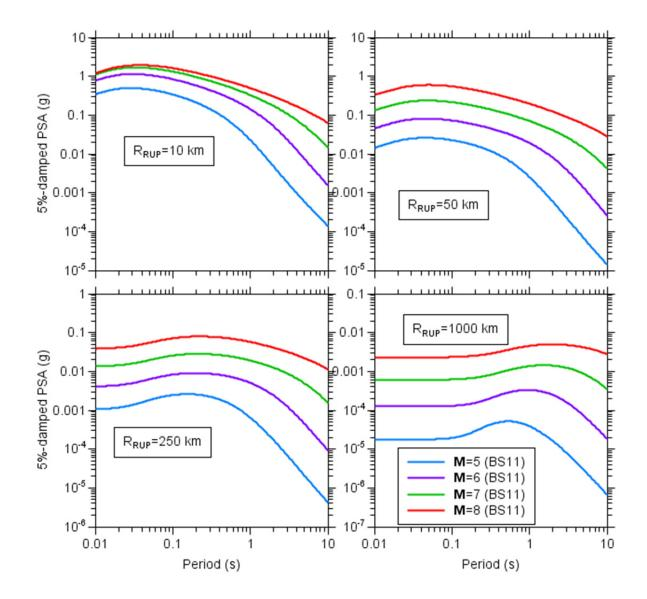
**Figure 2.23** Simulated 5%-damped response spectra for the Boatwright and Seekins [2011] (BS11) attenuation model as a function of period for four magnitudes and four distances. The Boore and Thompson [2015] finite-fault factor for stable continental regions was used to convert  $R_{RUP}$  to the distance  $R_{PS}$  used in the point-source simulations. The crustal amplifications used in the simulations were for sites with  $V_{S30} = 3.0$  km/sec.
