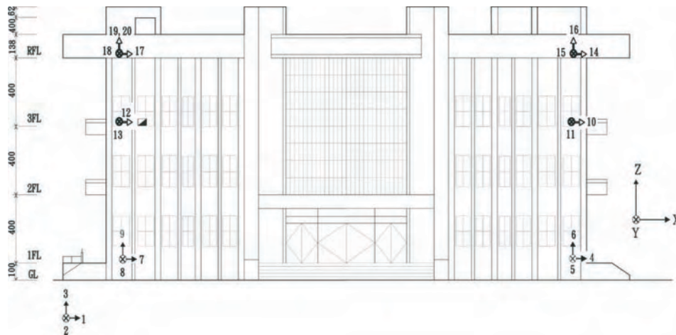
Fig. 16. Cross section view of the National Taitung Senior High Commercial and Vocational School where a strong-motion array is installed. The numbers in the left-hand side is in cm units, i.e., 4 m in height between different floors. The numbers (1 to 20) indicate where accelerometers are installed and correspond to the channel numbers in the Figs. 17 and 18.
